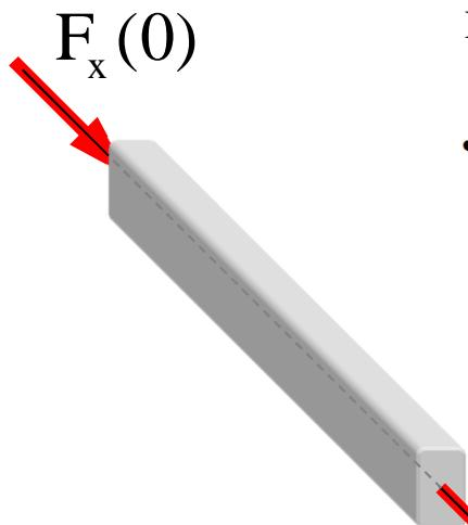
$$\int_0^L \frac{dN(x)}{dx} \bar{u}(x) dx = N(L) \bar{u}(L) - N(0) \bar{u}(0) - \int_0^L \frac{N(x) \bar{N}(x)}{EA} dx$$
