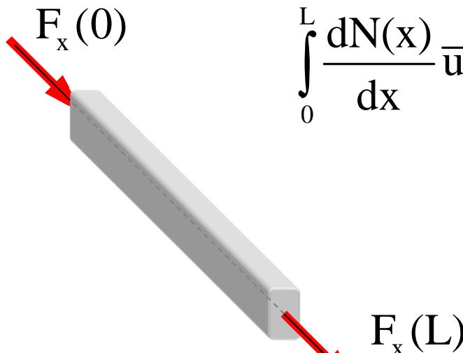
$$\int_0^L \frac{dN(x)}{dx} \bar{u}(x) dx = N(L) \bar{u}(L) - N(0) \bar{u}(0) - \int_0^L \frac{N(x) \bar{N}(x)}{EA} dx$$
