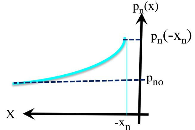
$$p'_n(x) = p'_n(-x_n) e^{-\frac{(x+x_n)}{L_p}} = [p_n(-x_n) - p_{n0}] e^{-\frac{(x+x_n)}{L_p}} = p_{n0} (e^{V/V_{Te}} - 1) e^{-\frac{(x+x_n)}{L_p}}$$
