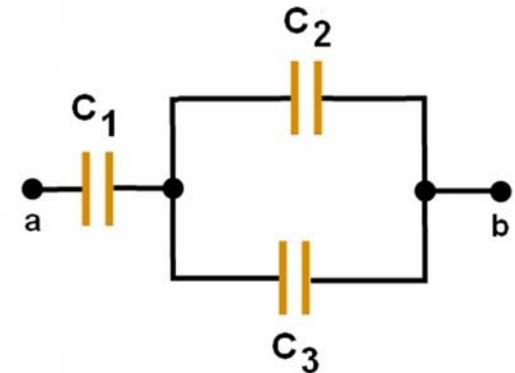
$$C_{eq} = \frac{C_1 (C_2 + C_3)}{C_1 + C_2 + C_3}$$
