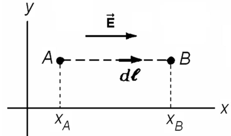
$$E_x = -\frac{\partial V}{\partial x} \quad E_y = -\frac{\partial V}{\partial y} \quad E_z = -\frac{\partial V}{\partial z}$$
