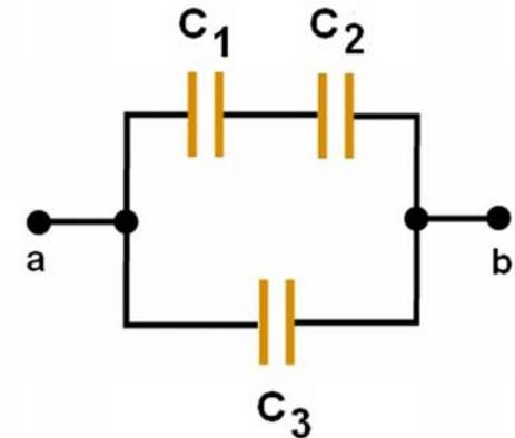
$$C_{eq} = \frac{C_1 C_2 + C_3 (C_1 + C_2)}{C_1 + C_2}$$
